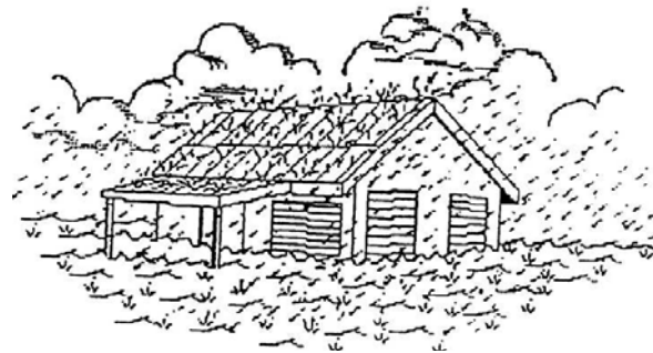
5.4 When cyclones are accompanied with heavy rain for a long duration, the buildings can be damaged due to flooding also. Building contents are spoiled due to rain when roofing sheets fly away.
