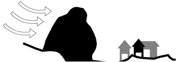
Shielding of house by hillock
